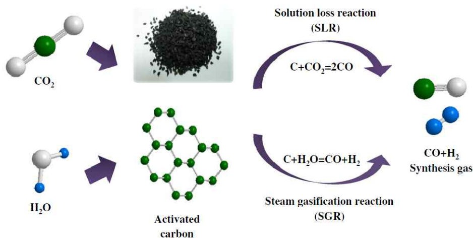
Fig. 1. A schematic of interaction among activated carbon, steam and carbon dioxide for syngas production.
