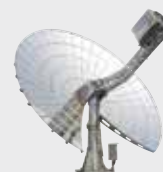
Dish type solar concentrator (10kWe)
