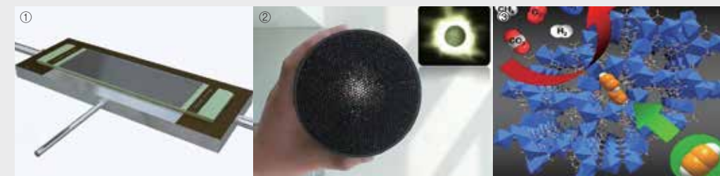
① SOEC stack for hydrogen mass production ② 300 CPSI C-SiC composite honeycomb for CSP ③ Gas separation using metal organic frameworks
