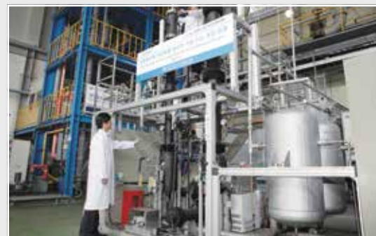
CO 2 recovery process using promoted K 2 CO 3 aqueous solution
