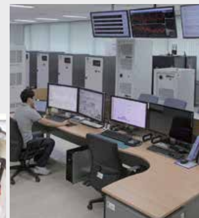
300 kVA real-time computer simulation system for microgrid
