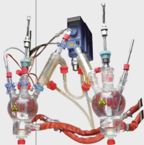
Different reaction calorimeter for analyzing heat of absorption
