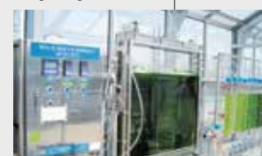
Photobioreactor system using sunlight and coal-firing flue gas
