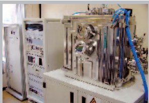
▲ EB-PVD 코팅 장치 및 ZrO 2 코팅된 디젤엔진 밸브 (Coating Equipment of EB-PVD and Coated Diesel Engine Valve with ZrO 2 )
