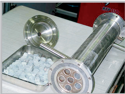
▲ 수증기개질 촉매 및 열교환형 반응기 (Monolith-type Steam Reforming Catalyst and Heat-exchanger Type Reactor)
