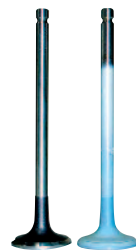
▲ EB-PVD 코팅 장치 및 ZrO 2 코팅된 디젤엔진 밸브 (Coating Equipment of EB-PVD and Coated Diesel Engine Valve with ZrO 2 )
