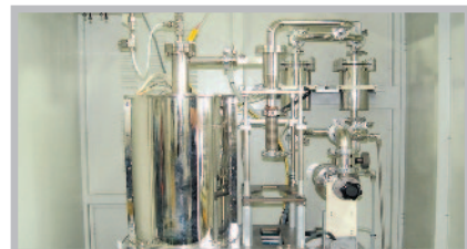
▼ Lab-scale 유동층 화학기상증착 장치 (Lab-scale Fluidized Bed Chemical Vapor Deposition Equipment)
