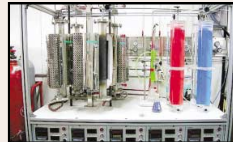
▲ 20 L/hr 급 IS 사이클 수소생산 장치(Hydrogen Production by IS(Iodine-Sulfur) Process(20 L/hr)) ◆ 50 L/hr 급 열화학적 물분해 수소 제조 장치(Hydrogen Production by Thermochemical Water-splitting(50 L/hr))
