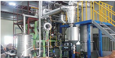
Rapid Pyrolysis Process for Lignocellulosic Biomass (Capacity : 2tons/day)
