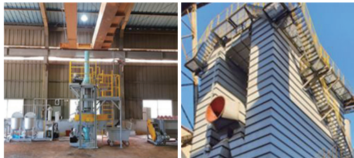
Low Ash Biomass Manufacturing Facility (11ton/day) Filter Dust Collector with 1/10 Dust Discharge
