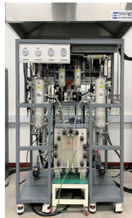
Alkaline Water Electrolysis Stack for Responding to Load Variation
