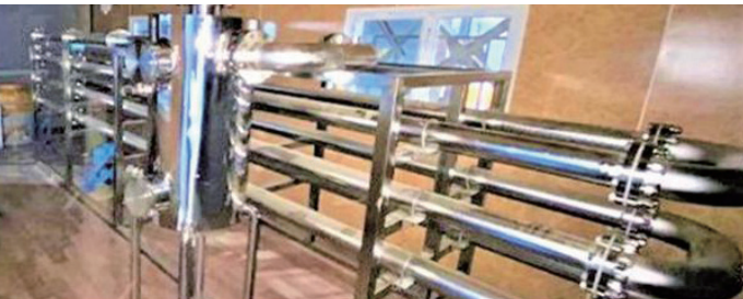
Simultaneous CO 2 Capture-Mineralization System (100kg-CO 2 /day)
