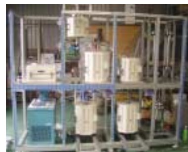
▲ 초청정석탄 제조장치 (Preparation of Ash-Free Coal)
