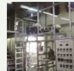
◀ PVC 함유 페플라스틱의 탈염장치 (Screw Reactor System for the Dechlorination of PVC Containing Waste Plastics) ▼ 고분자 폐기물 열분해 유화 실증 플랜트 (Demonstration Plant for the Pyrolysis of Polymer Wastes)
